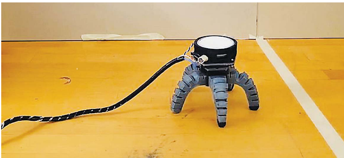
Natural electrical signals in the mushroom that are triggered by light are able to power the hybrid device's insect-style legs.
