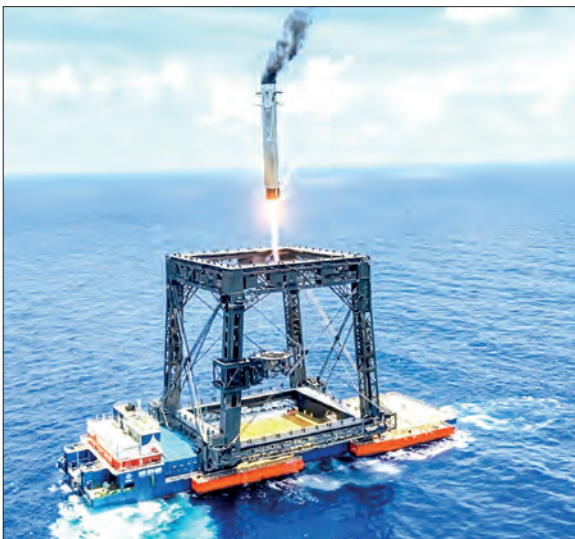
A video grab shows a platform mounted on the recovery ship Linghangzhe successfully capturing the first-stage booster of the Long March 10B carrier rocket on Friday. PHOTO: CCTV
