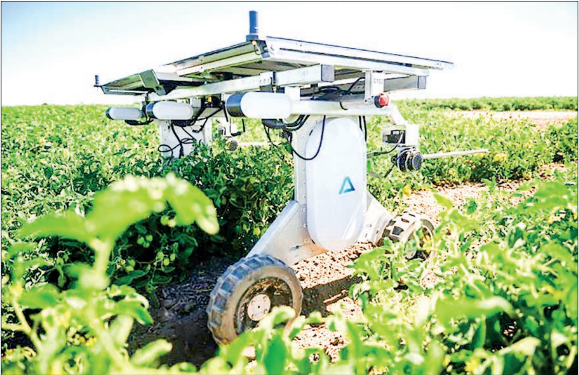
Aigen's solar-powered autonomous robots aim to take the chemicals and toil out of industrial weeding. PHOTO: AFP
